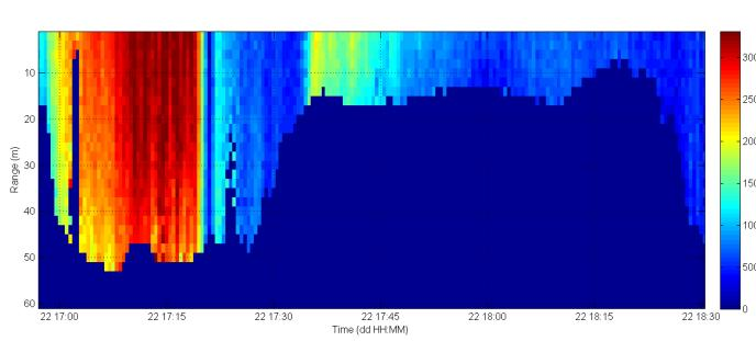
**ADCP data** measured flow velocity, to ground truth UAV measurements.
