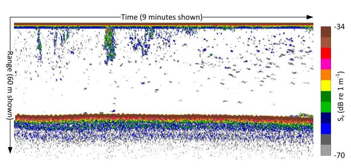
**EK60** data measured fish schools and turbulence characteristics, to link to UAV images of surface characteristics.
