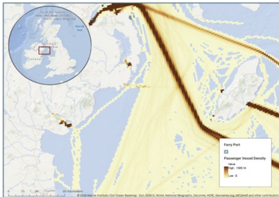
Figure 8 | Passenger vessel density and ferry ports in the Western Irish Sea. Passenger vessel density, with darker shades of red indicating areas of higher density and lighter shades of yellow representing lower density. Ferry ports are also highlighted. This visualisation identifies areas of intensive shipping activity, informing where to place offshore wind farms to avoid major disruption.
