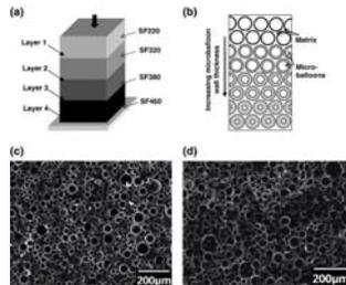
Advanced processing methods are being developed to introduce compositional gradients into various material systems, including core materials, e.g. syntactic foams.
